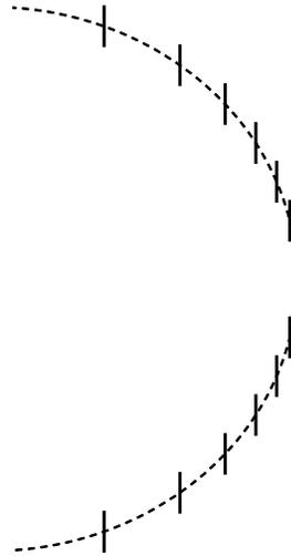
Figure 10. Cross-section of stator divided into concentric rings of *equal width*, where purely for illustration each ring has been shifted to the left by the distance that a wave would have travelled during the time delay applied to that ring.
