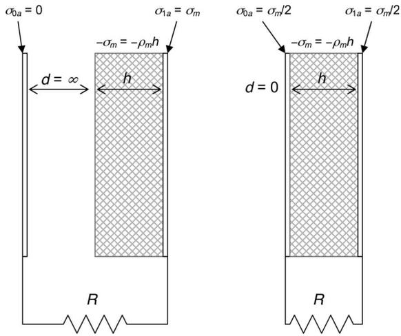
FIG. 3. Induced electrode charge at  $d=0$  and  $d=\infty$ .
