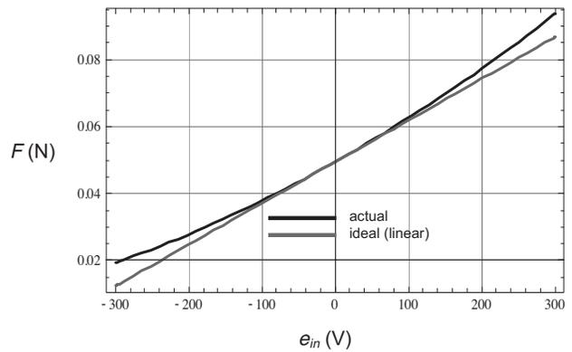
FIG. 6. Linearity of force vs voltage of single-ended transducer with membrane blocked where  $S = \pi a^2$ , where  $a = 15$  mm,  $d = 200$   $\mu\text{m}$ ,  $h = 12$   $\mu\text{m}$ ,  $\sigma_m = 14.1$  mC/m<sup>2</sup>,  $\epsilon_0 = 8.85$  pF/m,  $\epsilon_r = 12$ , and  $\epsilon_{r1} = 1$ .
