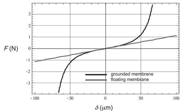
FIG. 5. Linearity of force vs displacement of push-pull transducer with input shorted where  $S = \pi a^2$ , where  $a = 15$  mm,  $d = 200$   $\mu\text{m}$ ,  $h = 12$   $\mu\text{m}$ ,  $\sigma_m = 14.1$  mC/m<sup>2</sup>,  $\epsilon_0 = 8.85$  pF/m,  $\epsilon_r = 12$ , and  $\epsilon_r = 1$ .
